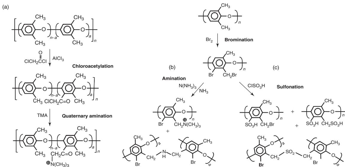
**Figure 6.9** Main reactions and structures of IEMs from PPO: (a) anion exchange membranes employing Friedel-Crafts chloroacetylation, (b) anion exchange membrane prepared by bromination and amination, and (c) cation exchange membrane prepared by bromination and sulfonation reaction.
