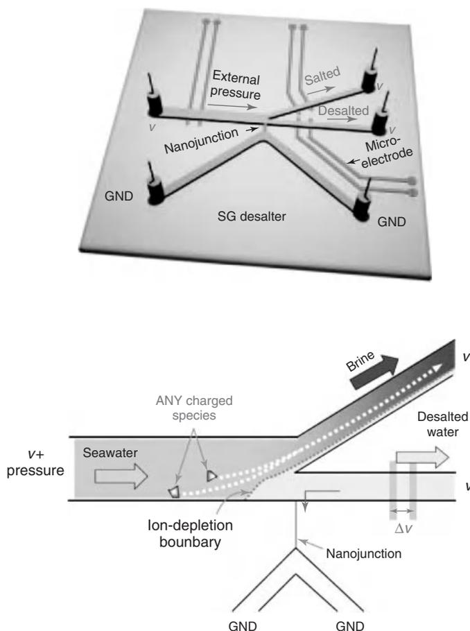
**Figure 6.16** ICP desalination scheme: (a) micro/nanofluidic desalination system with embedded microelectrode for the measuring potential drop and (b) electrokinetic desalination operation associated with the external pressure [156].
