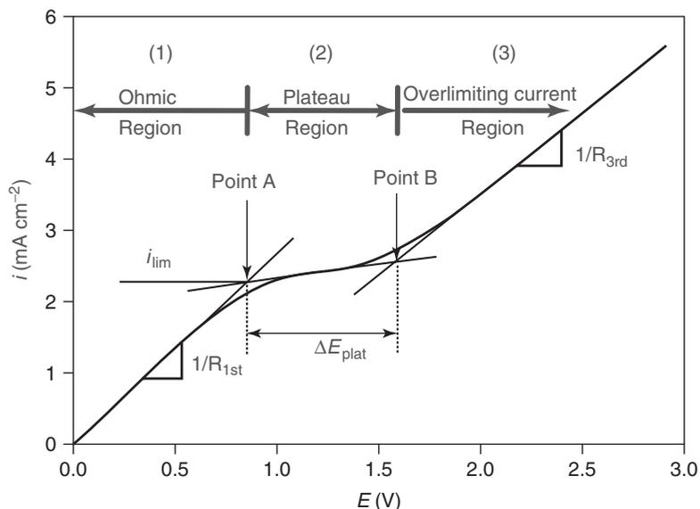
**Figure 6.4** The representative characteristic  $i$ - $v$  curve.
